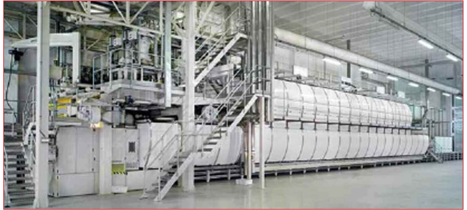
Pasta dryers are modular designed and contain 4 to 10 climate zones.
